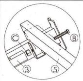
2.2 Place the centre rail (4) into its corresponding "U" shaped brackets on the width bars (5). Tightly secure the centre bar using the 1/4"x40mm screw (B) and Nut(C).
