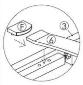
3.1 Insert the slats (6) into the end slat cap (F) and fix it to the corresponding holes on the side rail.
