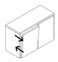
**Depth Adjustment**after loosening the hinge arm mounting screw
